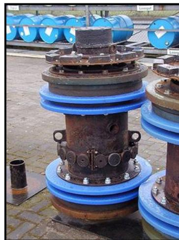
**Figure 2:** ‘Pig’ used to clean out pipelines.
